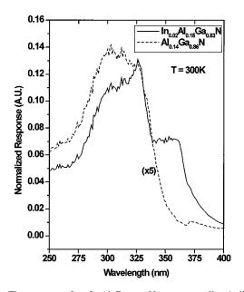
FIG. 3. The response of an  $In_xAl_yGa_{1-x-y}N$  quaternary alloy (solid line) and  $Al_yGa_{1-y}N$  alloy (dotted line) with comparable cutoff wavelength. The compositions for these samples are estimated to be  $In_{0.02}Al_{0.15}Ga_{0.83}N$  and  $Al_{0.14}Ga_{0.86}N$ , respectively.
