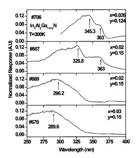
FIG. 2. Normalized photoresponse VS wavelength of incident light of  $In_xAl_yGa_{1-x-y}N$  quaternary alloys with different In and Al contents. The arrows indicate the cutoff wavelength for the quaternary alloys. The photoresponse from the underlying GaN epilayer in the two samples Nos. 706 and to P 667 is seen in the steps at 363 nm.
