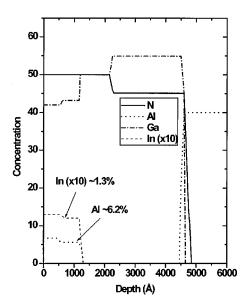
FIG. 1. Rutherford backscattering (RBS) analysis of  $In_xAl_yGa_{1-x-y}N$  quaternary alloy grown on top of GaN epilayer (No. 706). This sample is found to contain 1.3% indium and 6.2% aluminum (atomic composition). This is close to the composition predicted theoretically for lattice matching to GaN (x:y=1:4.7).
